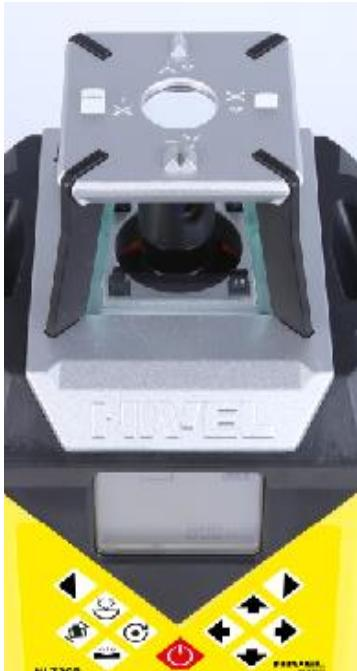
Enter into manual mode by pressing key on the keypad. Set up X axis slope manually by press or . Set up Y axis slope manually by press & . See at the laser head value of slope direction (+/-).
